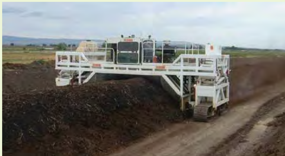
Compost turner. Turning the compost oxygenates the rows and speeds up the process
